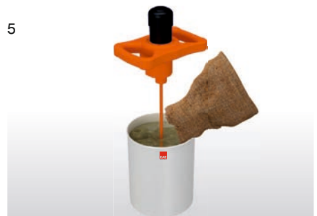
Add fillers and mix until homogeneous; at least 5 minutes. Then application must be done within 15 minutes.
